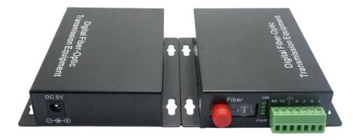
Fiber modem implements advanced optic transmission technology to extend signal transmission distance up to 120km on single-core fiber. It can convert data type among RS232, RS422 and RS485 by one circuit or multi-circuit. With features of HV-free,electromagnetic-free and thunder-lightning protection, fiber modem is widely used in industrial control, automatic electricity system, and traffic control etc.
